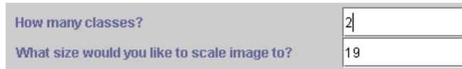
Figure G.25: Classes details tab of Image Data File Creator application: This is the first tab of the application. The first text box specifies how many different classes are going to be used in the problem. This number will set the appropriate number of text boxes needed on the second tab to enter the locations of the directories containing the images for each class.
